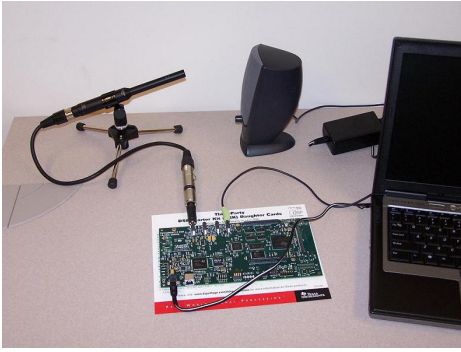
Figure 2: The DSP based prototype for acoustic OFDM modem
